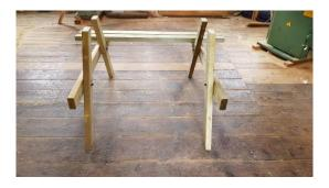
Fix the second A frame leg to the other end of the seat section you have just fitted using 2 x 100mm bolts, washers and nuts.
