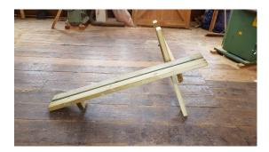
Bolt together one of the A frame legs to one of the seat sections using 2 x 100mm bolts. Add the washer and nut.
