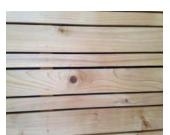
Renowned for its high decay resistance, though it is not resistant to insect attack, this wood varies in colour and shade, typically a reddish to pinkish brown. It is lightweight and stable; and is an attractive timber that is easy to work with.
