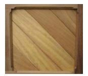
This is a very durable wood ideal for use outdoors. It is initially a stripy yellow / orange but darkens to a richer brown over time, and is a fantastic wood for timber gates and planters. It is especially resistant to rot, insect or fungus attack and can be a low cost alternative to teak at times.
