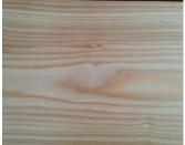
It is a great all-rounder with its popularity increasing as it is specified more by architects and landscapers, due to its strength and durability. It is a tough softwood and ideal for items where physical damage may occur for example gates, fence posts and other exterior applications (cladding, bridges, decking etc.) or where there is going to be ground contact.
