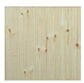
Contrary to its name this wood isn't red! It is brown with a reddish tint. It comes in different grades for different uses and knots are common in this timber. Boards vary in width from 100mm – 225mm.
